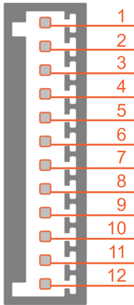
Digital in connector: pin-out (terminal block male)
