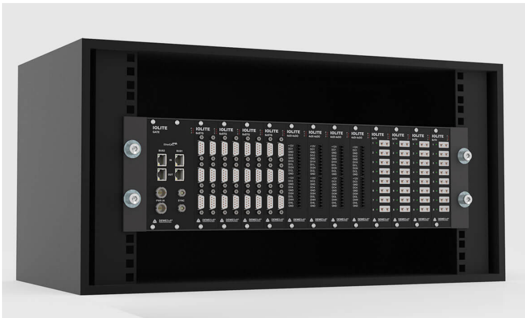
Mounting of IOLITE-R12 in the 19" cabinet
