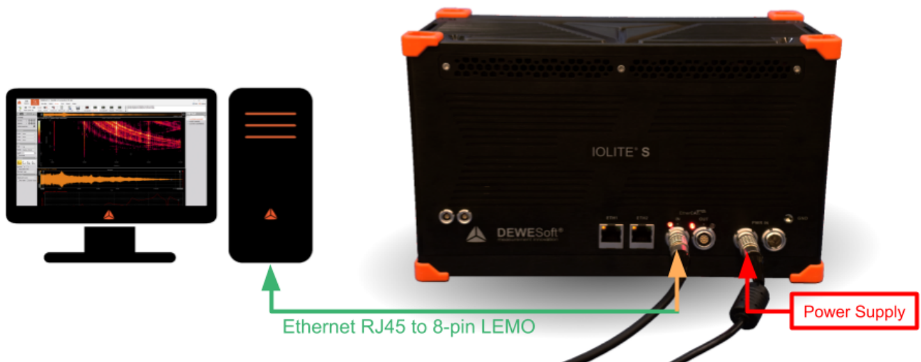
Connection of IOLITE-R8 standalone device to PC
