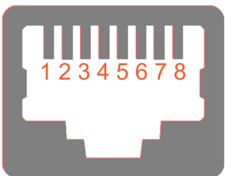
EtherCAT connector: pin-out (RJ-45 female)
