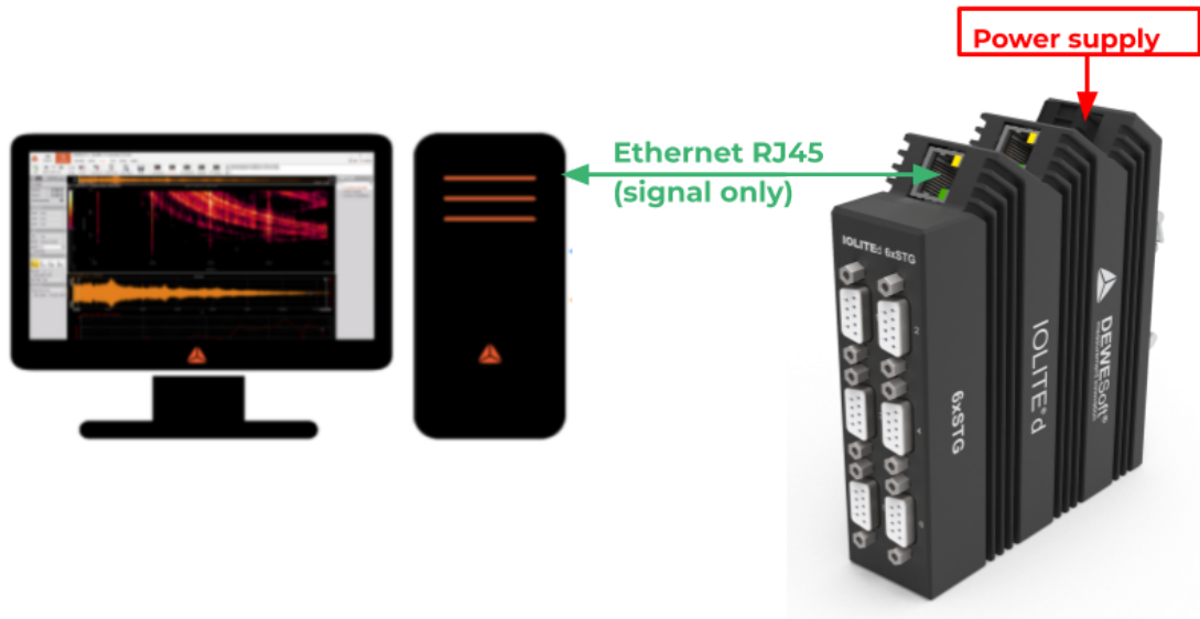
Connection of IOLITEi multi-channel standalone device to PC
