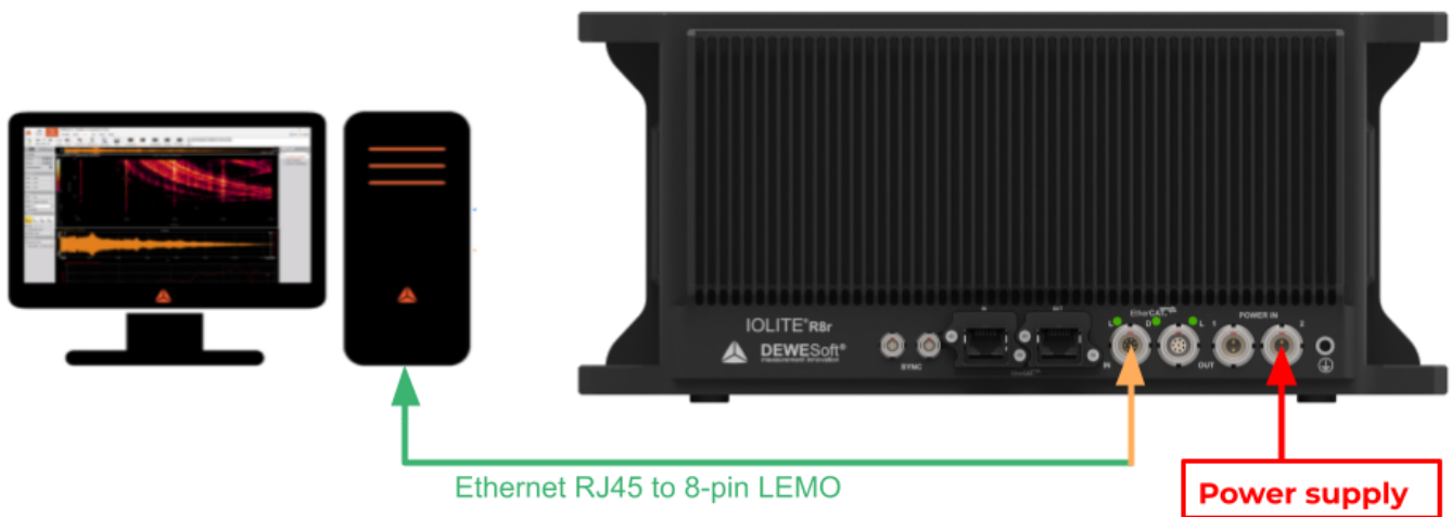
Connection of IOLITE-R8r standalone device to PC
